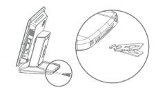
1.Insert locking clip into the designated slot located at the back of the stand
