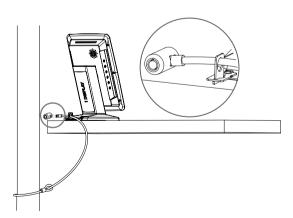
4.Insert the security cable through the slot and lock the cable
