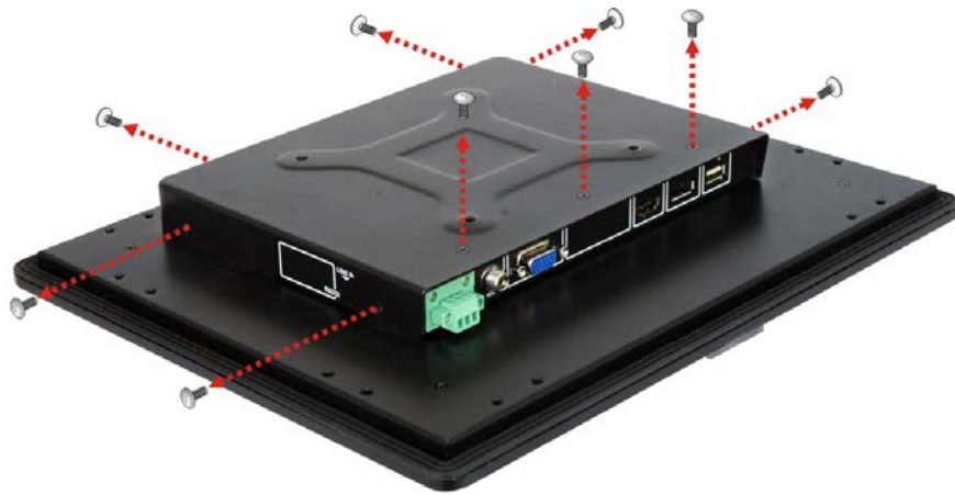
Figure 3-10: Rear Panel Retention Screw Removal (DM-F12A ~ DM-F24A)
