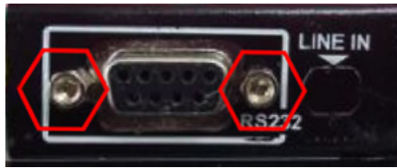
Figure 3-12: Hex Jack Screws for Securing RS-232 Connector
